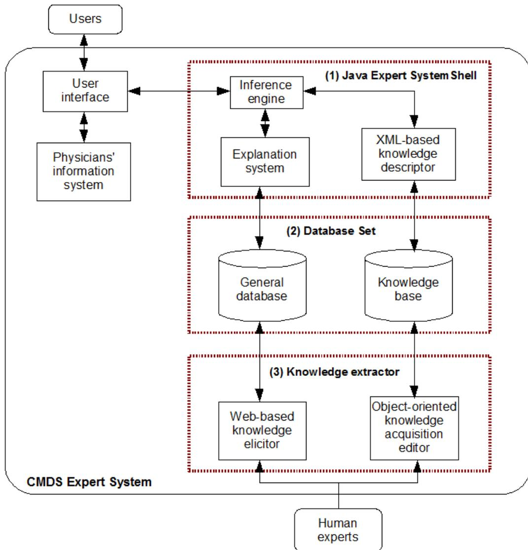
Figure 18: CMDS architecture (modified from Huang et al., 2007)
