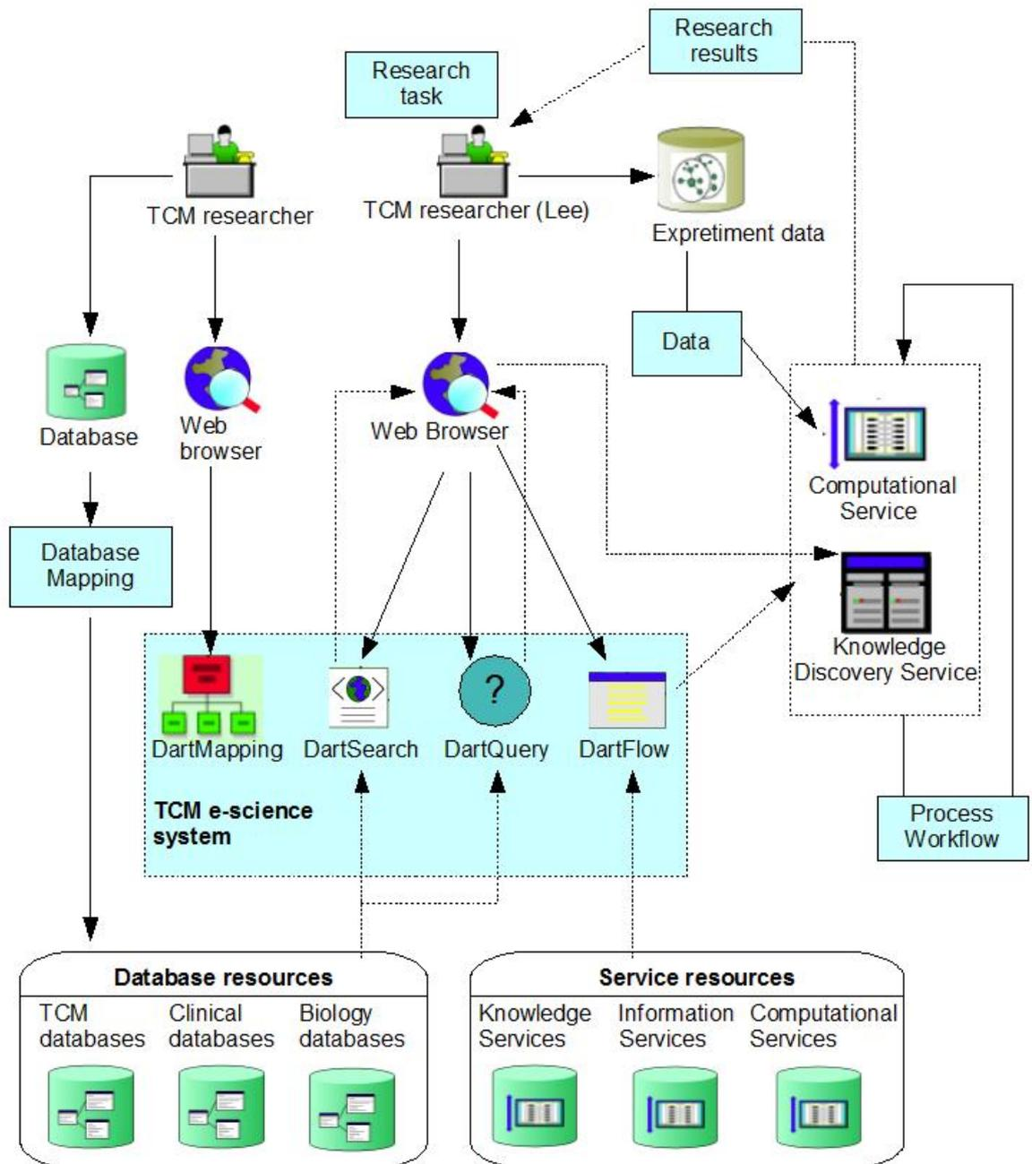
**Figure 23: A scenario of using the TCM e-science system for research (modified from Chen et al., 2007)**
