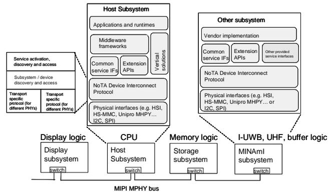
Figure 3. MINAmI subsystem NoTA extension architecture
