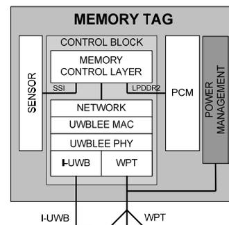
Figure 6. MINAmI architecture on a RF memory tag
