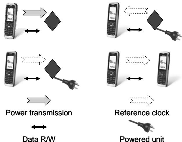
Figure 15. Some possible operational combinations of mobile phones interacting with MINAmI memory tags.
