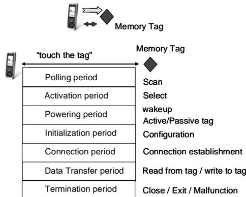
Figure 9. Mobile reader/writer to RF memory tag communication sequence
