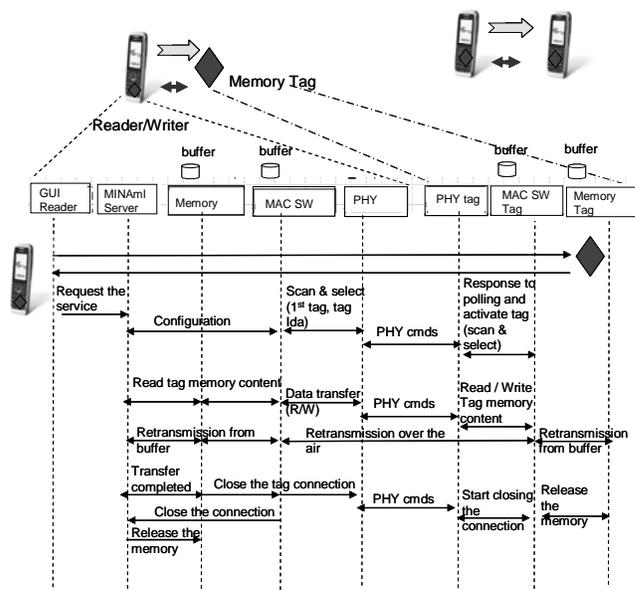
Figure 10. Basic MINAmI subsystem communication setup sequence
