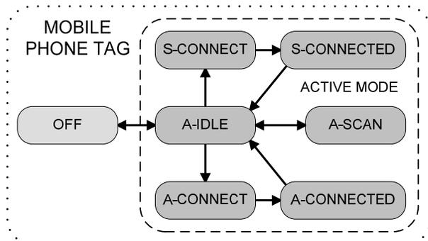
Figure 7. Active (and semi-passive) UWBLEE MAC states on a mobile phone. Active states denoted with A, semi-passive with S.
