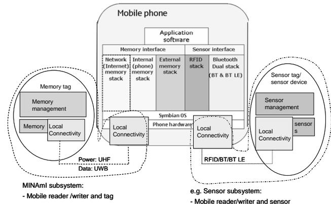
Figure 4. MINAmI architecture and MINAmI subsystem evolving towards NoTA compatibility.
