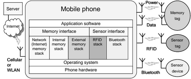
Figure 1. MINAmI Architecture. The Bluetooth stack includes both Classic Bluetooth and Bluetooth Low Energy profiles. On a sensor device side only either Classic BT or BT Low Energy stack is needed.
