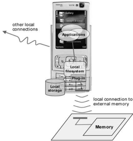
Figure 11. File system view of a mobile phone reading a passive memory tag: a cheap tag without its own processor.
