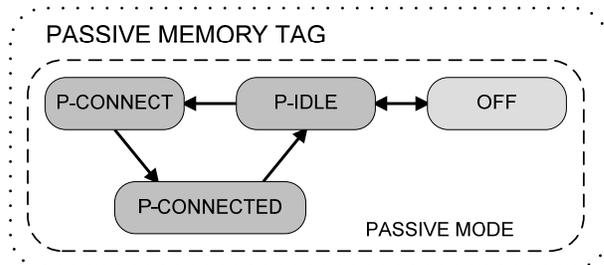
Figure 8. Passive UWBLEE MAC states on a RF memory tag.
