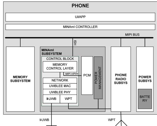
Figure 5. MINAmI architecture on a phone
