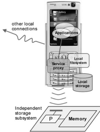
Figure 12. File system view of a mobile phone reading a passive memory tag: a more expensive tag with its own processor.
